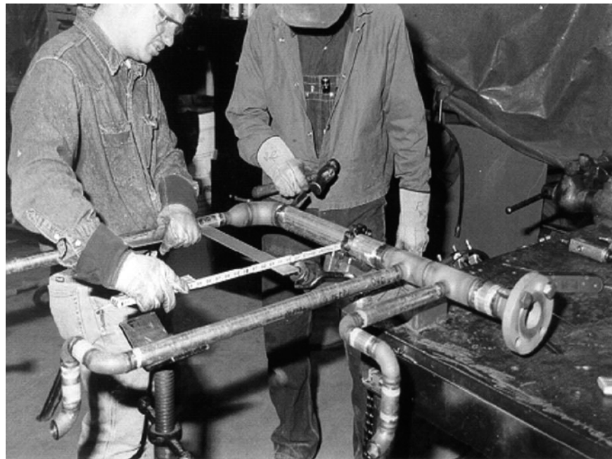
Figure 9.2 Weld fit-up and gap examples. (Photograph courtesy of TEAM Industries, Inc., Kaukauna, WI.)
